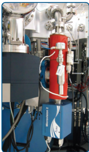
Microvision 2 installed as a 300mm Resist-Torr on a PVD tool degas chamber
